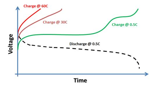
**Figure 5**. Charge/discharge profiles of the **Flash Battery** containing the multifunctional electrode (MFE) design
