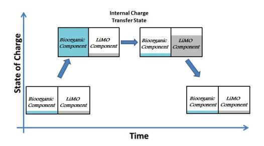
**Figure 4.** Charging mechanism of the multifunctional electrode structure
