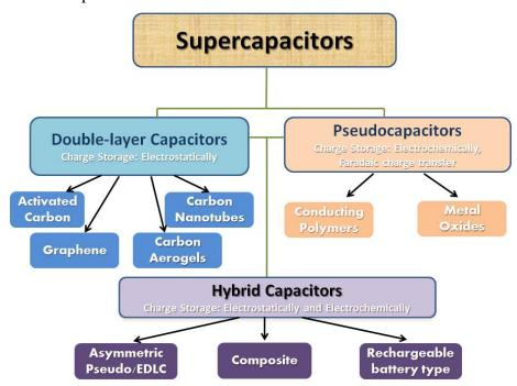
Figure 2. Hierarchical classification of supercapacitors and related types
