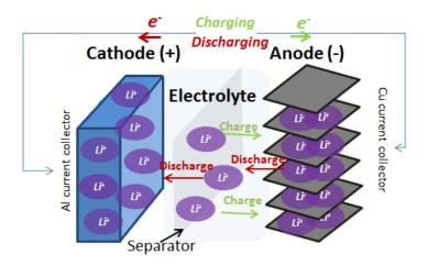
Figure 1. Lithium-ion battery structure
