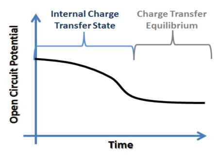
Figure 6. Relaxation mechanism inside the multifunctional electrode structure
