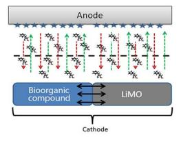
**Figure 8**. Schematic structure of **Flash Battery** containing multifunction electrode and organic compounds on the surface of the anode (stars) and inside the electrolyte
